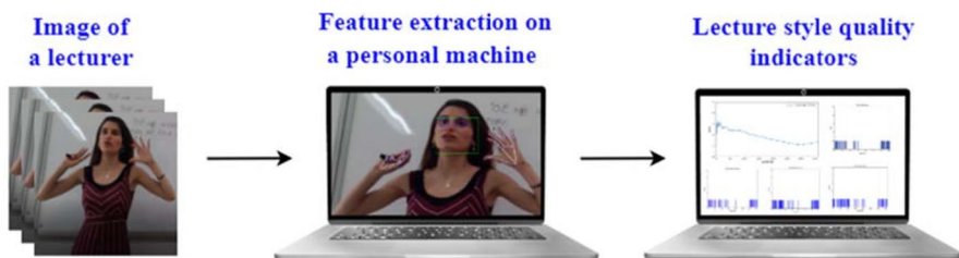
Fig. 1 Automated BLA tool. A video of a lecture captured by an ordinary camera is analysed to extract body language quality indicators
